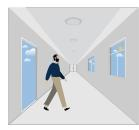
With sufficient daylight, the sensor keeps light OFF even motion gets detected.
