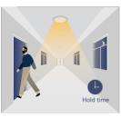
After there's no motion detected, the sensor keeps light ON 100% for holdtime.
