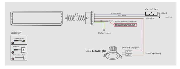
Emergency Driver can be used with either a switched or unswitched or emergency only fixture. If a switched fixture is used, an unswitched hot lead must be connected to the emergency driver.
